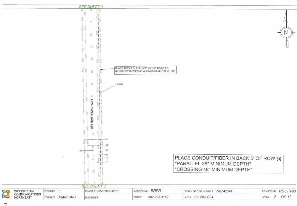
PLACE CONDUIT/FIBER IN BACK 5' OF ROW @ "PARALLEL 36" MINIMUM DEPTH" "CROSSING 48" MINIMUM DEPTH"
