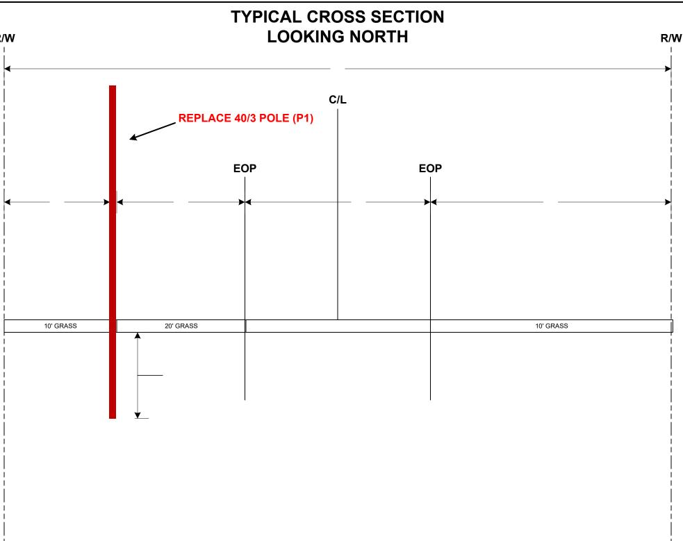
Note: Unknown depths will need to be determined at the time of construction via pothole.
