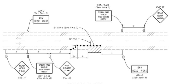
:TWO-LANE ROADWAY === SHOULDER WORK LESS THAN 2' FROM THE TRAVELED WAY WITH WORK ZONE SPEED OF 45 MPH OR LESS
