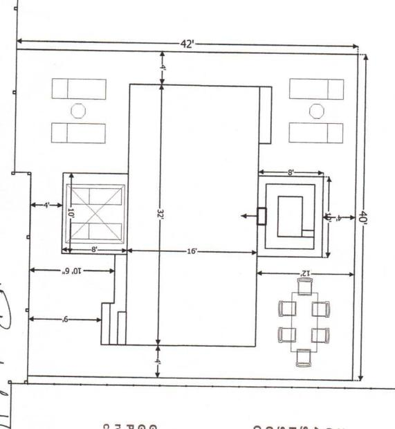
Concrete Deck w/ Kooldeck Surface Salt System Sunledge 18" Deep w/Umbrella Anchor Color Lights Pool Vac 400,000 BTU LP Gas Heater 6'x 8' Spa raised 18" 16'x 32' Pool 3 1/2'- 6'Deep
