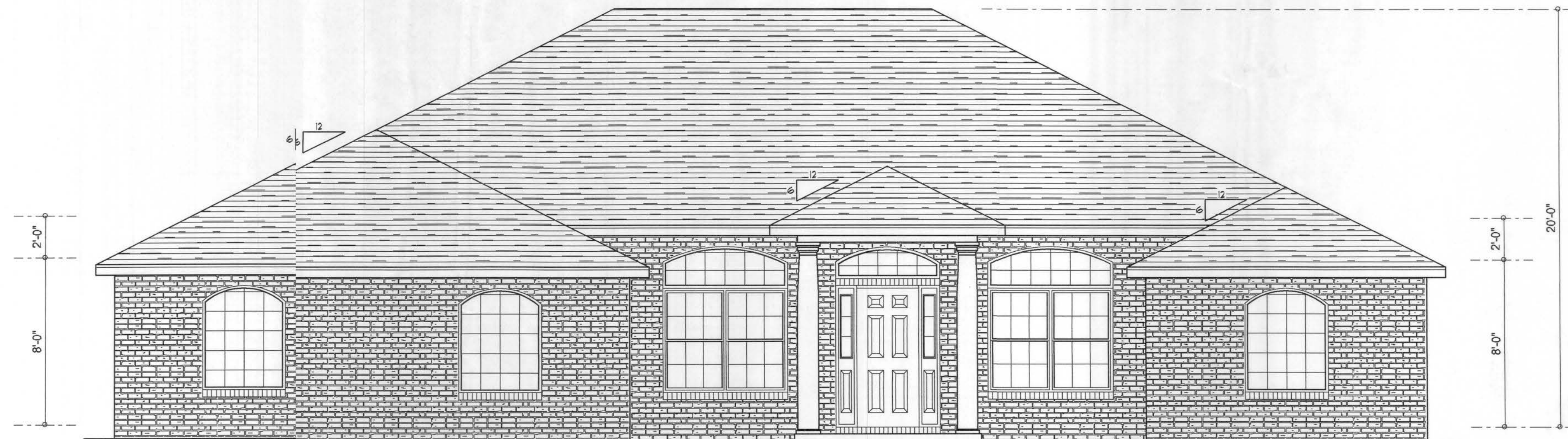
FRONT ELEVATION SCALE: 1/4" = 1'-0"
