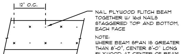
PLYWOOD FLITCH BEAM DETAIL
