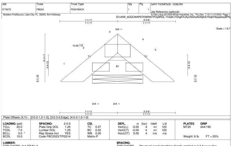
TOP CHORD 2x4 SP No.2 BOT CHORD 2x4 SP No.2 TOP CHORD **BOT CHORD**  Structural wood sheathing directly applied or 2-3-6 oc purlins. Rigid ceiling directly applied or 6-0-0 oc bracing.
