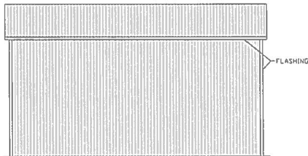
TYPICAL SIDE ELEVATION VERTICAL ROOF/SIDING OPTION
