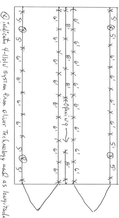
(8) indicates 4-11010 system from plicer Technology used as longitudual Devicus only, X indicates I Beam piers 6'QC. using 17x25 ABS PAdS assuming loso # 50:1.
