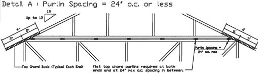
Piggyback cap truss stant nailed to all top chord purin bracing with (2) 16d box neis (0.135"x3.5") and secure top chord with 2x4 0.3 grade scab (1 side only at each end) attached with 2 rows of 10d box neis (0.126"x3") at 4" o.c.
