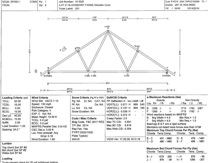
Truss passed check for 20 psf additional bottom chord live load in areas with 42"-high x 24"-wide
