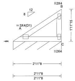
▲ Maximum Reactions (lbs), or \*=PLF Loc R /U /Rw /Rh /RL /W C\* 81 /2 /54 /- /11 / 35.5 Wind reactions based on MWFRS Min Brg Width Req = Bearing A is a rigid surface.
