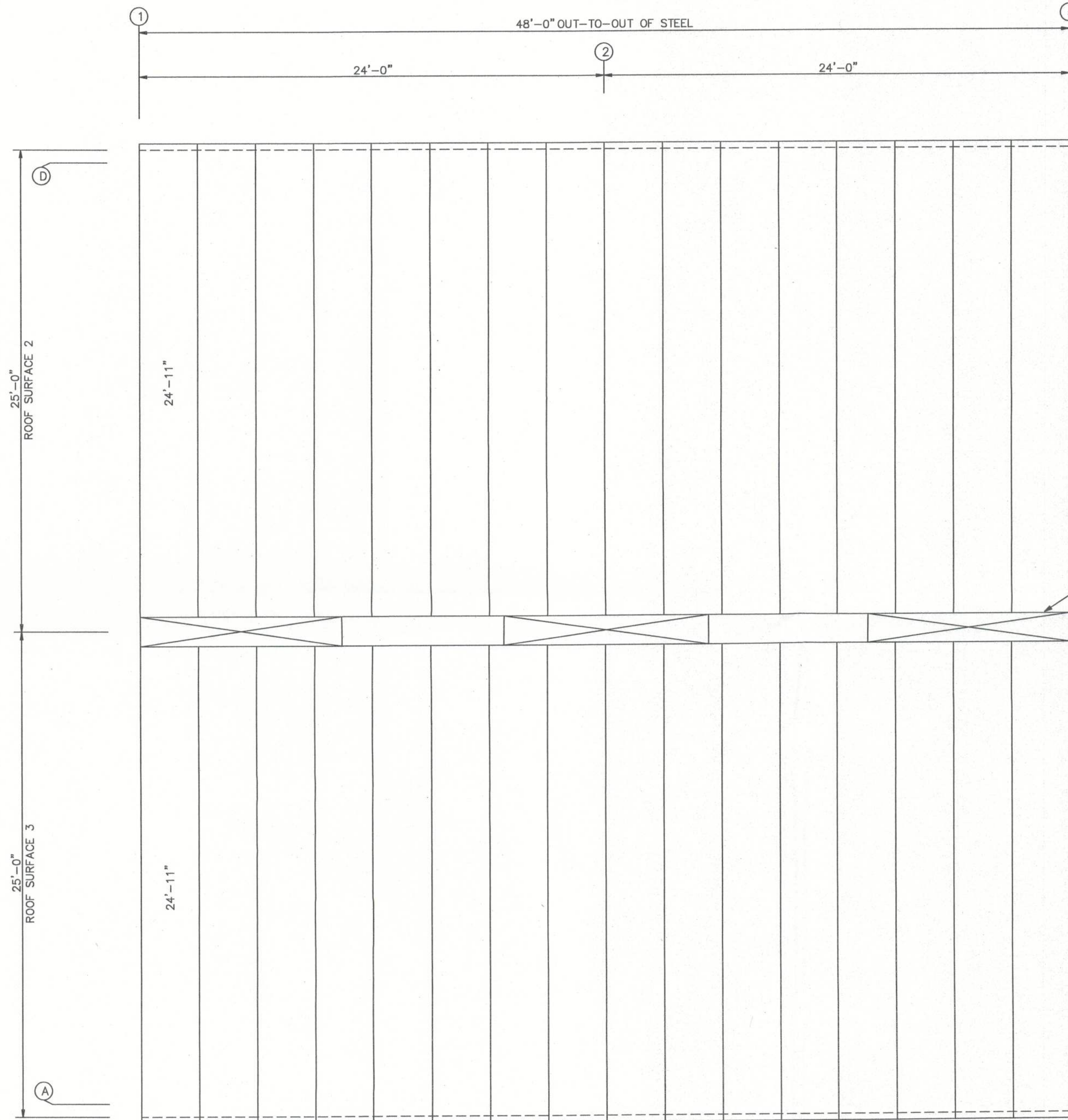
ROOF SHEETING PLAN PANELS: 26 Ga. PBR - Galvalume
