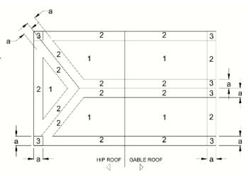
a: 10% OF LEAST HOIZONTAL DIMENSION OR 0.4%, WHICHEVER IS SMALLER, BUT NOT LESS THAN BITHER AN OF LEAST HORIZONTAL DIMENSION OR 3FT (0.9M). OR AS DETERMINED BY DESIGN OR OTHER APPLICABLE CODE.
