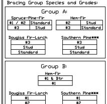
1x4 Braces shall be SRB (Stress-Rated Board). \*\*\*\*For 1x4 So. Pine use only Industrial 55 or Industrial 45 Stress-Rated Boards. Group B values may be used with these grades.
