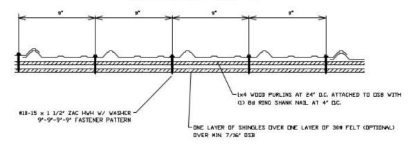
MINIMUM 29 GA. CAPITAL RIB PANEL PANEL SYSTEM TYPE 2 FASTENER PATTERN AT 24" O.C.
