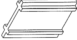
MEDIUM MULLION REINFORCEMENT #20634 ALUMINUM 6063-T6
