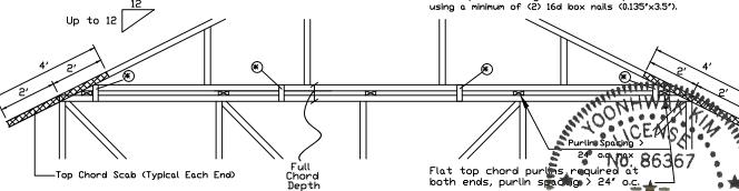
Note: If purlins or sheathing are not specified on the flat top of the bose truss, purlins must be installed at 24" o.c. max. and use Detail A.
