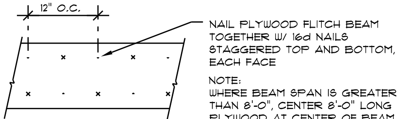
PLYWOOD FLITCH BEAM DETAIL
