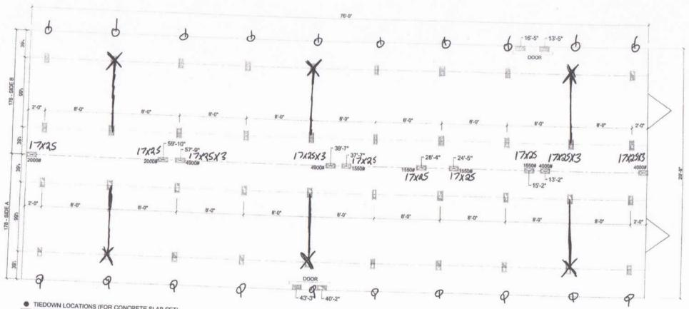
TIEDOWN LOCATIONS (FOR CONCRETE SLAB SET) MARRIAGE LINE OPENING SUPPORT PIER/TYP.
