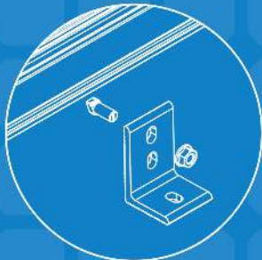
INTEGRATED BONDING MICROINVERTER MOUNT w/ WIRE MANAGEMENT
