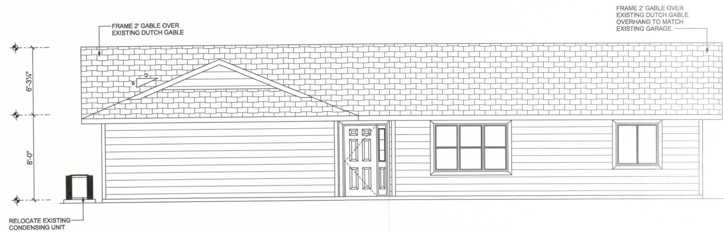
PROPOSED FRONT ELEVATION SCALE: 3/16" = 1'-0"
