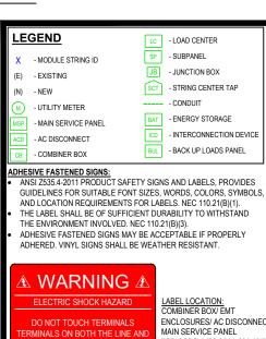
ENCLOSURES/ AC DISCONNECT/ MAIN SERVICE PANEL PER CODE: NEC 2017, 690.13(B)
