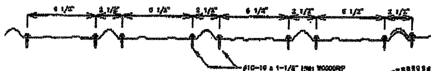
FASTENER PATTERN TYPE B, AT 12" O.C.
