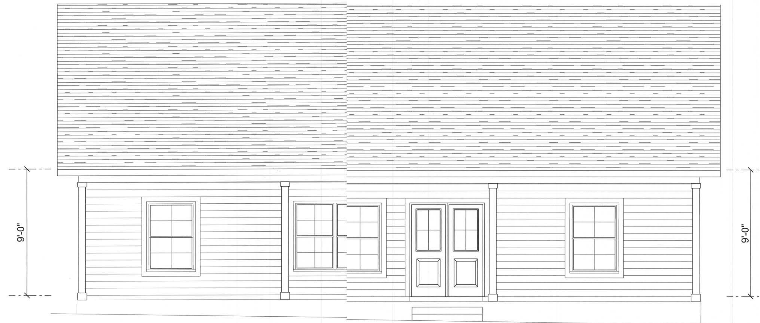
FRONT ELEVATION SCALE: 1/4" = 1'-0"
