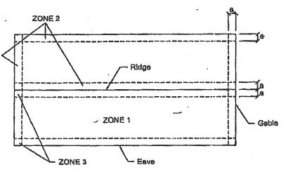
Note: Dimension (a) is defined as 10% of the minimum width of the building or 40% of the mean height of the roof, whichever is amaller, however, (e) cannot be less than either 4% of the minimum width of the building or 3 feet.
