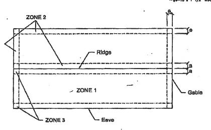
Note: Dimension (a) is defined as 10% of the minimum width of the building or 40% of the mean height of the roof, whichever is amaller, however, (a) cannot be less than either 4% of the minimum width of the building or 3 feet.
