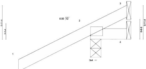
Plate Offsets (X,Y)-[2:Edge,0-0-3] LOADING (psf) SPACING-2-0-0 CSI. DEFL in I/defl L/d **PLATES** GRIP 244/190 TCLL 20.0 Plate Grip DOL 1.25 TC 0.32 Vert(LL) 0.00 >999 240 MT20 TCDL 7.0 Lumber DOL 1.25 вс 0.09 Vert(CT) 0.00 >999 180 **BCLL** 0.0 Rep Stress Incr YES WB 0.00 Horz(CT) 0.00 2 n/a n/a BCDL 10.0 Code FBC2017/TPI2014 Matrix-MP Weight: 7 lb FT = 20%
