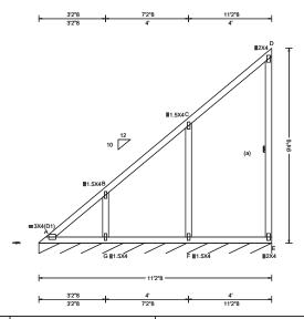
Loading Criteria (psf) TCLL: 20.00 TCDL: 10.00 BCLL: 0.00 BCDL: 10.00 Des Ld: 40.00 NCBCLL: 10.00 Soffit: 2.00 Load Duration: 1.25 Spacing: 24.0 "
