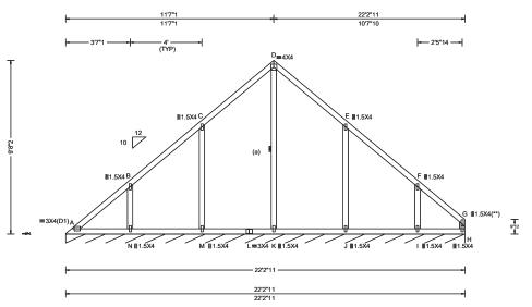
Loading Criteria (psf) TCLL: 20.00 TCDL: 10.00 BCLL: 0.00 BCDL: 10.00 Des Ld: 40.00 NCBCLL: 10.00 Soffit: 2.00 Load Duration: 1.25 Spacing: 24.0 "
