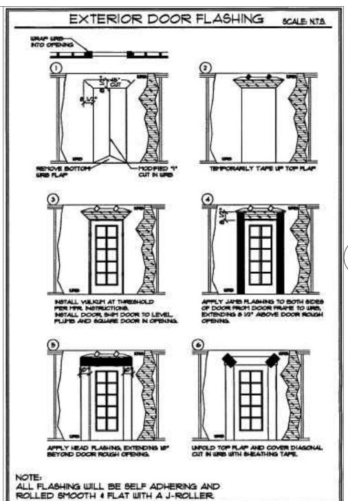
NOTE: THESE DETAILS USED FOR DOORS & WINDOW. ALL FLASHING TO MEET FBC R903.2.1, R905.2.8. & R703.8 AND INSTALLED PER MANUFACTURER'S RECOMMENDATIONS.
