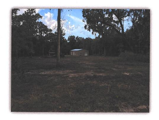
The elevation of the road adjacent to the site is 134.00 + /-. The highest existing ground elevation at the foundation is 4.5' below the existing road or 129.50 + /-. The minimum finished floor of the home will be 1.5' above the highest existing ground elevation or 131.00. The finished floor of the home will be below the nearest adjacent street.
