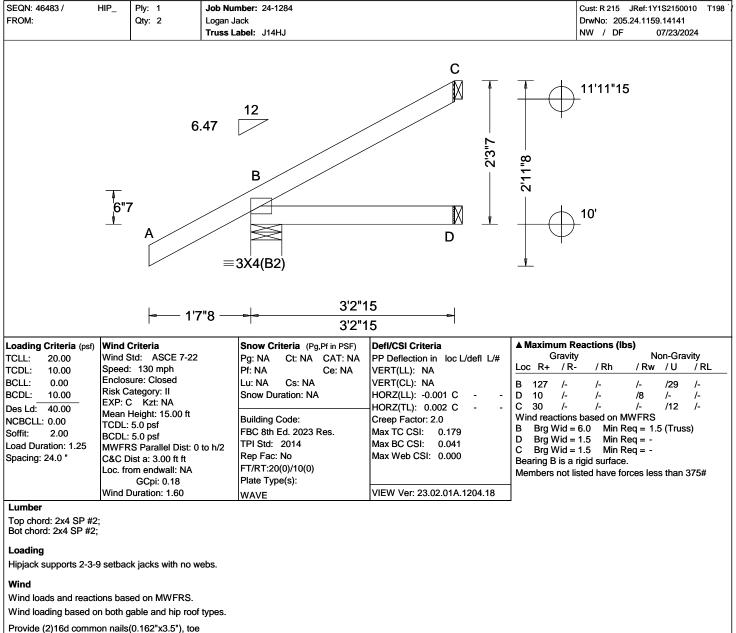
nailed at Top chord. Provide (2)16d common nails(0.162"x3.5"), toe nailed at Bot chord.
