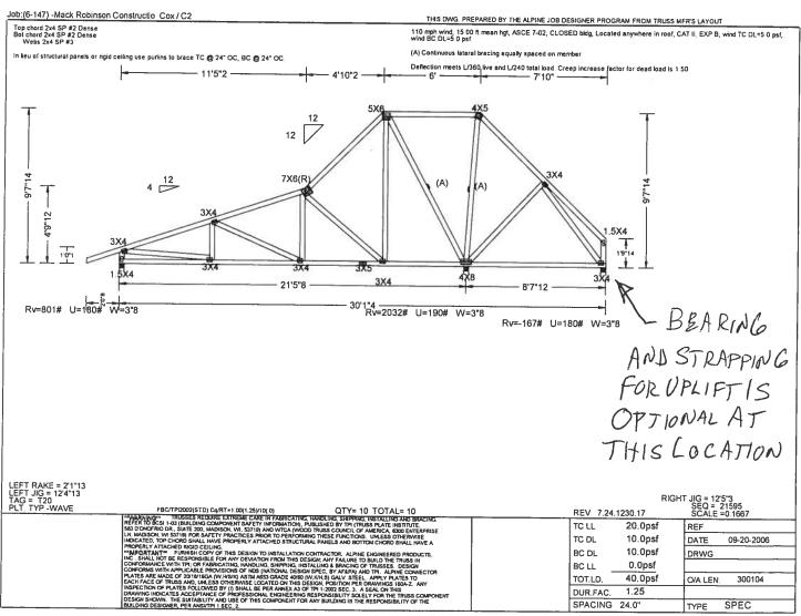
ADDENDUM TO PLAN TO ALLOW BEARING VSTRAPPING AT 30'1"4. THE TRUSS IS DESIGNED TO CANTALEVER BUT IT WORKS FOR ALL LOAD CASES IF IT BEARS ON WALL
