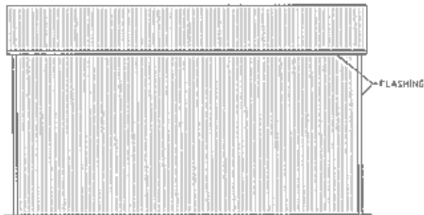
TYPICAL SIDE ELEVATION VERTICAL ROOF/SIDING OPTION
