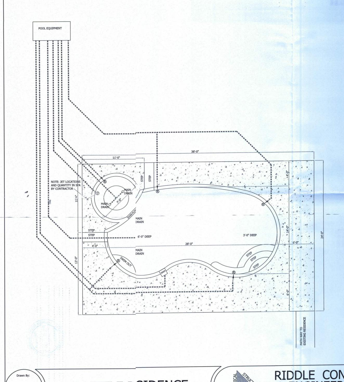
NOTE: IF ANY PART OF THE POOL **ENCROACHES UPON THE ANGLE OF** REPOSE, PLACE STEEL @ 6" o.c. EA WAY IN AREAS OF QUESTION
