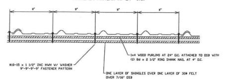
MINIMUM 29 GA. CAPITAL RIB PANEL PANEL SYSTEM TYPE 2 FASTENER PATTERN AT 24" O.C.
