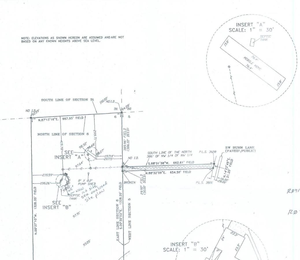
SYMBOL LEGEND 4"X4" CONCRETE MONUMENT FOUND 4\*X4\* CONCRETE MONUMENT SET IRON PIPE FOUND IRON PIN AND CAP SET POWER POLE WATER METER CENTERLINE SATELLITE DISH TELEPHONE BOX ---E--- ELECTRIC LINES SCALE: 1'' = 200'---- CHAIN LINK FENCE ---- WOODEN FENCE
