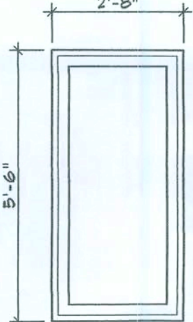
TYPE F ALUMINUM CASEMENT IMPACT RESISTANT RATED
