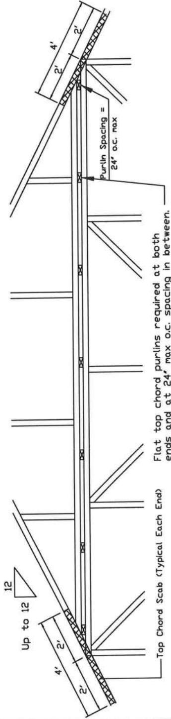
Piggyback cap truss slant nailed to all top chord purlin bracing with (2) 16d box nails (0.135"x3.5") and secure top chord with 2x4 #3 grade scab (1 side only at each end) attached with 2 rows of 10d box nails (0.128"x3") at 4' o.c.
