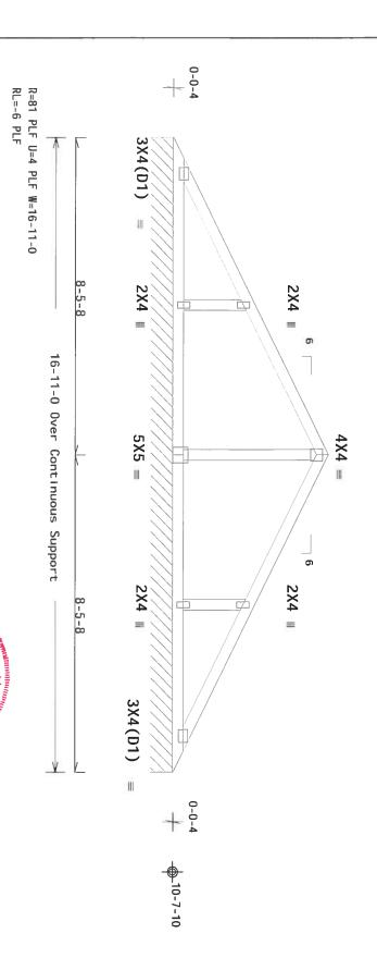
2400 Lake Orange Dr. Suite 150 Orlando, FL 32837 FL COA #0 278 AN ITW COMPANY Alpine, a division of INW Building Components Group Inc. shall not be responsible for any deviation drawing, any failure to build the truss in confermance with ANSI/TP1 1, or for handling, shipping, installation & bracing of trusses. for more information see this job's general notes page and these web sites: www.spineite.com, TPI www.spinetc.org, WTCA www.sbcindustry.com, ICC www.iccssfe.org
