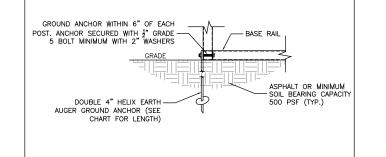
GROUND ANCHOR BASE RAIL DETAIL
