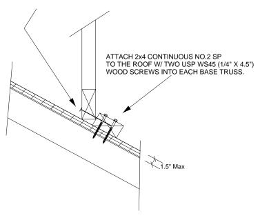
WIND DESIGN PER ASCE 7-98, ASCE 7-02, ASCE 7-05 146 MPH WIND DESIGN PER ASCE 7-10, ASCE 7-16 160 MPH MAX MEAN ROOF HEIGHT = 30 FEET ROOF PITCH = MINIMUM 3/12 MAXIMUM 6/12 CATEGORY II BUILDING EXPOSURE C WIND DURATION OF LOAD INCREASE: 1.60 MAX TOP CHORD TOTAL LOAD = 50 PSF MAX SPACING = 24" O.C. (BASE AND VALLEY)
