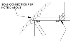
7" x 7" x 1/2" PLYWOOD (or 7/16" OSB) GUSSET EACH SIDE AT 24" O.C. ATTACH WITH 3 - 6d (0.113" X 2") NAILS INTO EACH CHORD FROM EACH SIDE (TOTAL - 12 NAILS)
