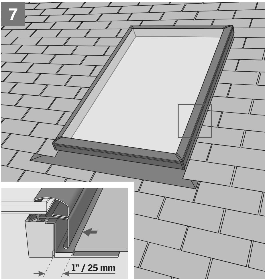
**ENGLISH:** Install asphalt shingles tight to sides and top of skylight.
