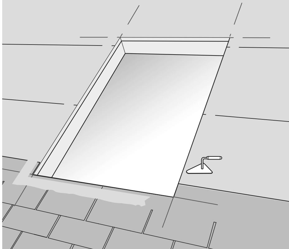
**ENGLISH:** Apply roof cement around the rough opening at all four sides.
