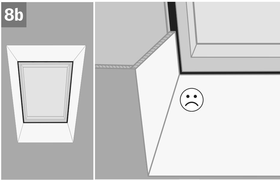
**ENGLISH:** When drywall is not in contact with white finished skylight frame, add on-site trim for finished appearance and to prevent conditions that may contribute to condensation.
