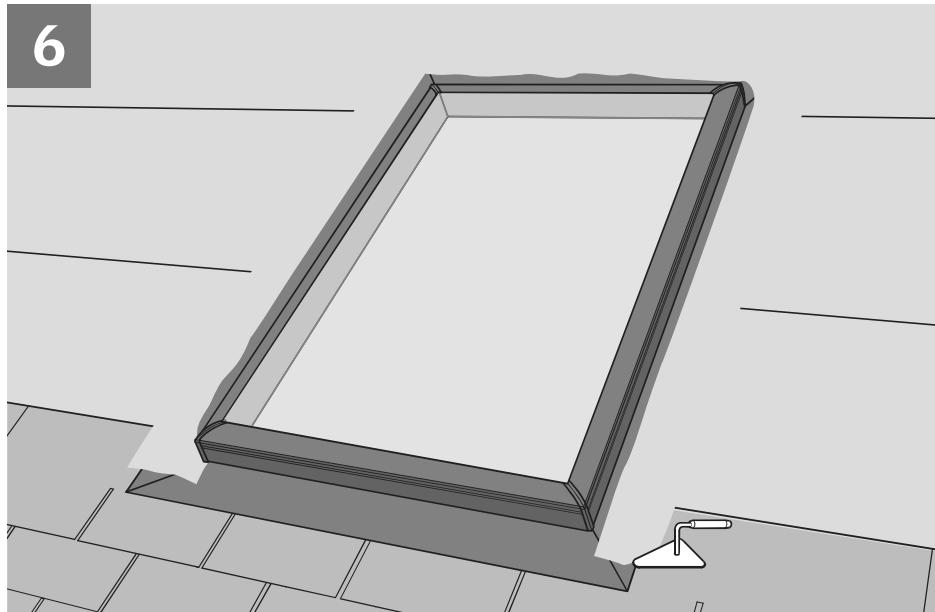
**ENGLISH:** Apply roof cement on flashing flange at sides and top.
