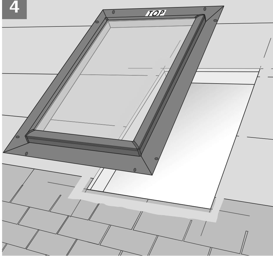
**ENGLISH:** Center the skylight over the rough opening by aligning the alignment marks on the flashing flange with the alignment corner lines at the rough opening. The skylight should be installed with a side labeled TOP pointing upwards.
