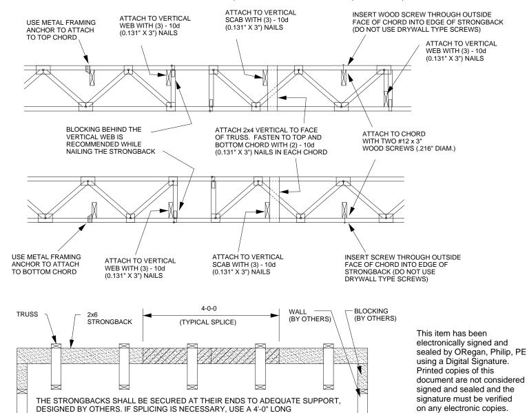
ALTERNATE METHOD OF SPLICING:
