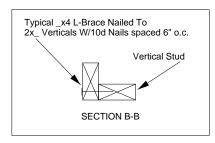
DIAGONAL BRACE TRUSS GEOMETRY AND CONDITIONS 4'-0" O.C. MAX SHOWN ARE FOR ILLUSTRATION ONLY. 12 Varies to Common Truss SEE INDIVIDUAL MITEK ENGINEERING DRAWINGS FOR DESIGN CRITERIA 3x4 =- Diagonal Bracing - L-Bracing Refer
