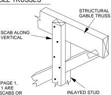
AN ADEQUATE DIAPHRAGM OR OTHER METHOD OF BRACING MUST BE PRESENT TO PROVIDE FULL LATERAL SUPPORT OF THE BOTTOM CHORD TO RESIST ALL OUT OF PLANE LOADS. THE BRACING SHOWN IN THIS DETAIL IS FOR THE VERTICAL/STUDS ONLY.
