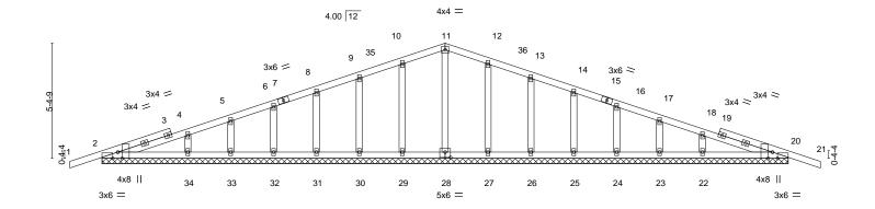
32-0-0 Plate Offsets (X,Y)--[2:0-3-8,Edge], [2:0-2-13,Edge], [20:0-2-13,Edge], [20:0-3-8,Edge], [28:0-3-0,0-3-0] SPACING-LOADING (psf) in (loc) I/defI L/d **PLATES** GRIP 1.25 TCLL 20.0 Plate Grip DOL TC 0.12 Vert(LL) -0.00 21 120 MT20 244/190 n/r TCDL 7.0 Lumber DOL 1.25 ВС 0.10 Vert(CT) -0.00 21 n/r 120 **BCLL** 0.0 Rep Stress Incr YES WB 0.05 Horz(CT) 0.00 20 n/a n/a Code FBC2020/TPI2014 FT = 20% **BCDL** 10.0 Weight: 162 lb Matrix-S
