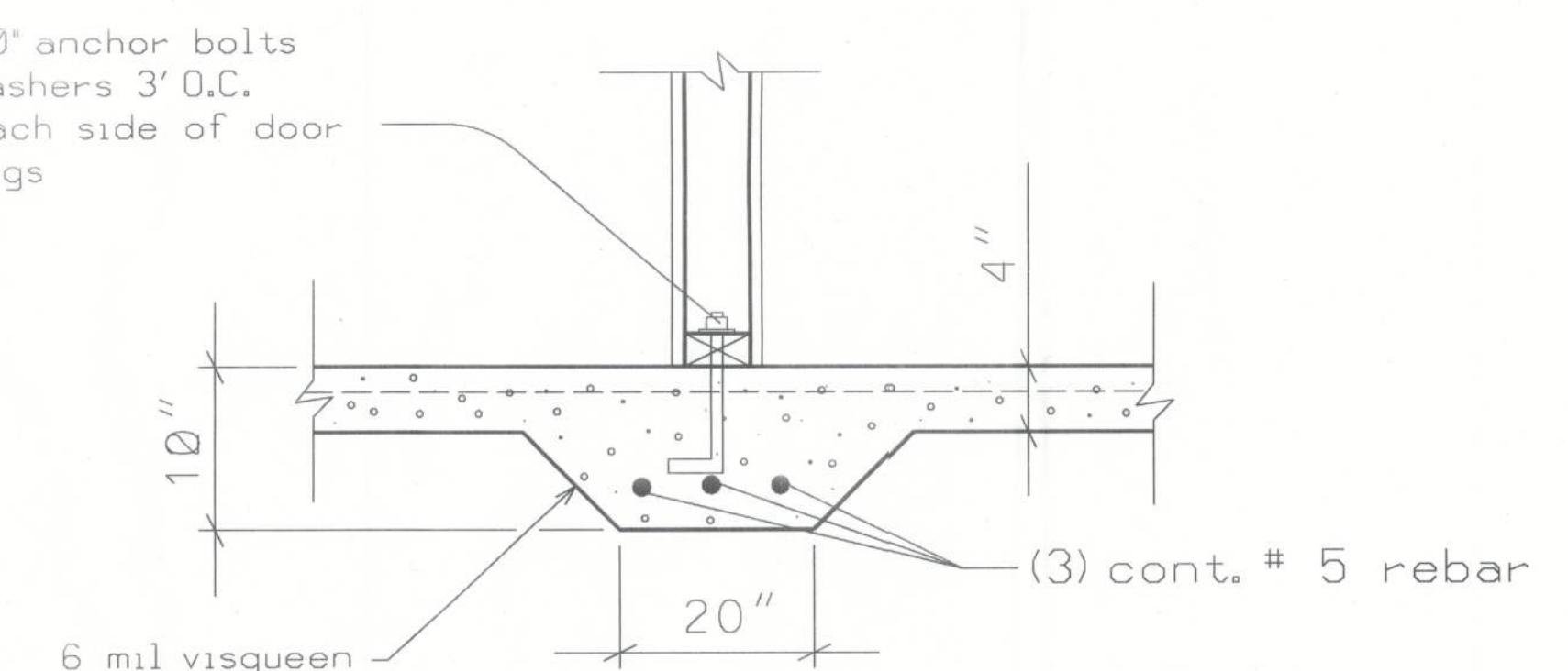
INTERIOR MONOLITHIC FOOTER DETAIL( N.T.S.)
