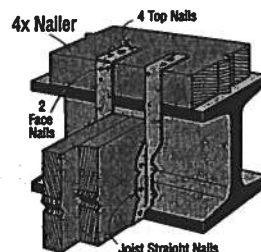
Typical THA Minimum Nailing Configuration on a 4x Nailer (except THA29)
