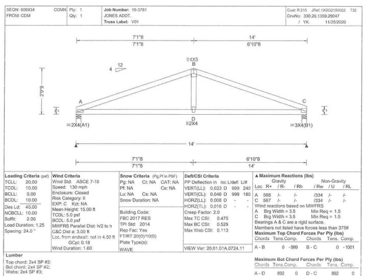
Wind loads based on MWFRS with additional C&C member design.
