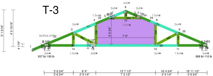
Max CSIs TC = LC: 25 (6-10) - 0.66 BC = LC: 16 (13-10) - 0.79 Web = LC: 2 (5-7) - 0.45 Max SSI = LC: 16 (6-10) - 0.62 Max Horizontal Deflection = 0.10" Max Vertical Deflection = 0.44" \$122.40 \$81.60 (Mat. Only)
