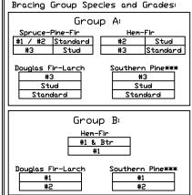
1x4 Braces shall be SRB (Stress-Rated Board) \*\*For 1x4 So. Pine use only Industrial 55 or Industrial 45 Stress-Rated Boards, Group B values may be used with these grades.
