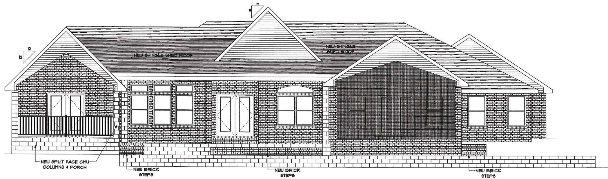
REAR ELEVATION SCALE: 1/4" = 1'-0"
