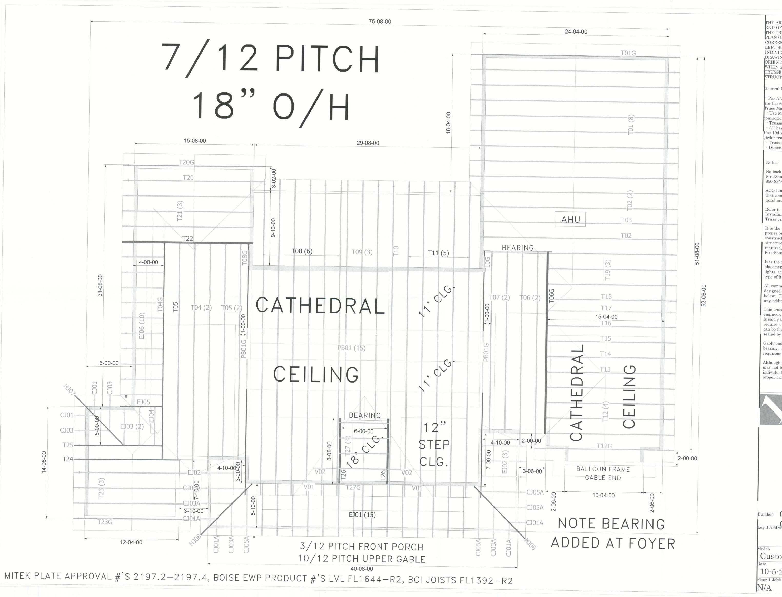
THE ARROW HEAD AT THE END OF THE TRUSS ON THE TRUSS PLACEMENT PLAN (LAYOUT) CORRESPONDS WITH THE LEFT SIDE OF THE INDIVIDUAL TRUSS DRAWING. USE THIS AS AN ORIENTATION GUIDE WHEN SETTING THE TRUSSES ON THE STRUCTURE.
