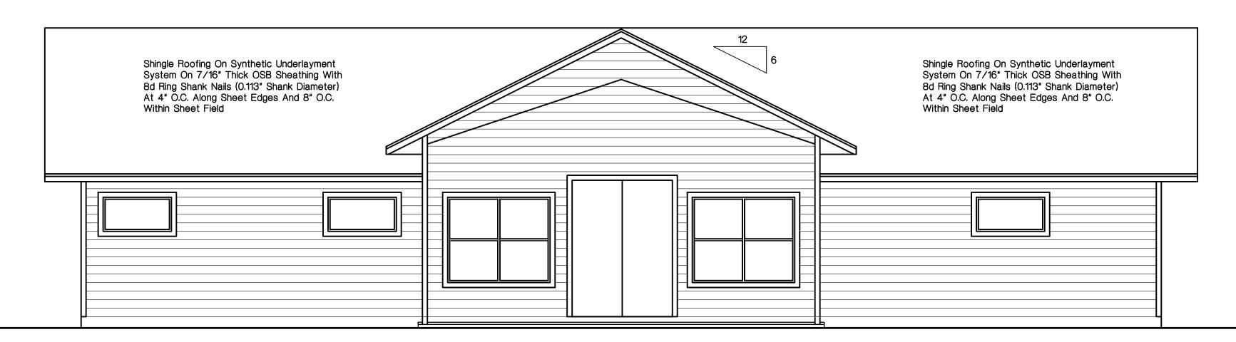
Finish Cement Lap Siding With 6" Lap Exposure Over Moisture Barrier On 7/16" OSB Wall Sheathing (NordBord Windstorm Wall Sheathing Or Equal) - Extend Wall Sheathing Vertical Or Horizontal From The Bottom Of The Bottom Plate With Continuous Load Path Up To The Top Of The Double Top Plate Install 2 x 4 Blocking At Horizontal Joint No Less Than 24" From Double Top Plate Or Bottom Plate With 8d Ring Shank (0.113" Shank Diameter) Nails At 3" Along Sheet Edges And 6" O.C. In Sheet Field
