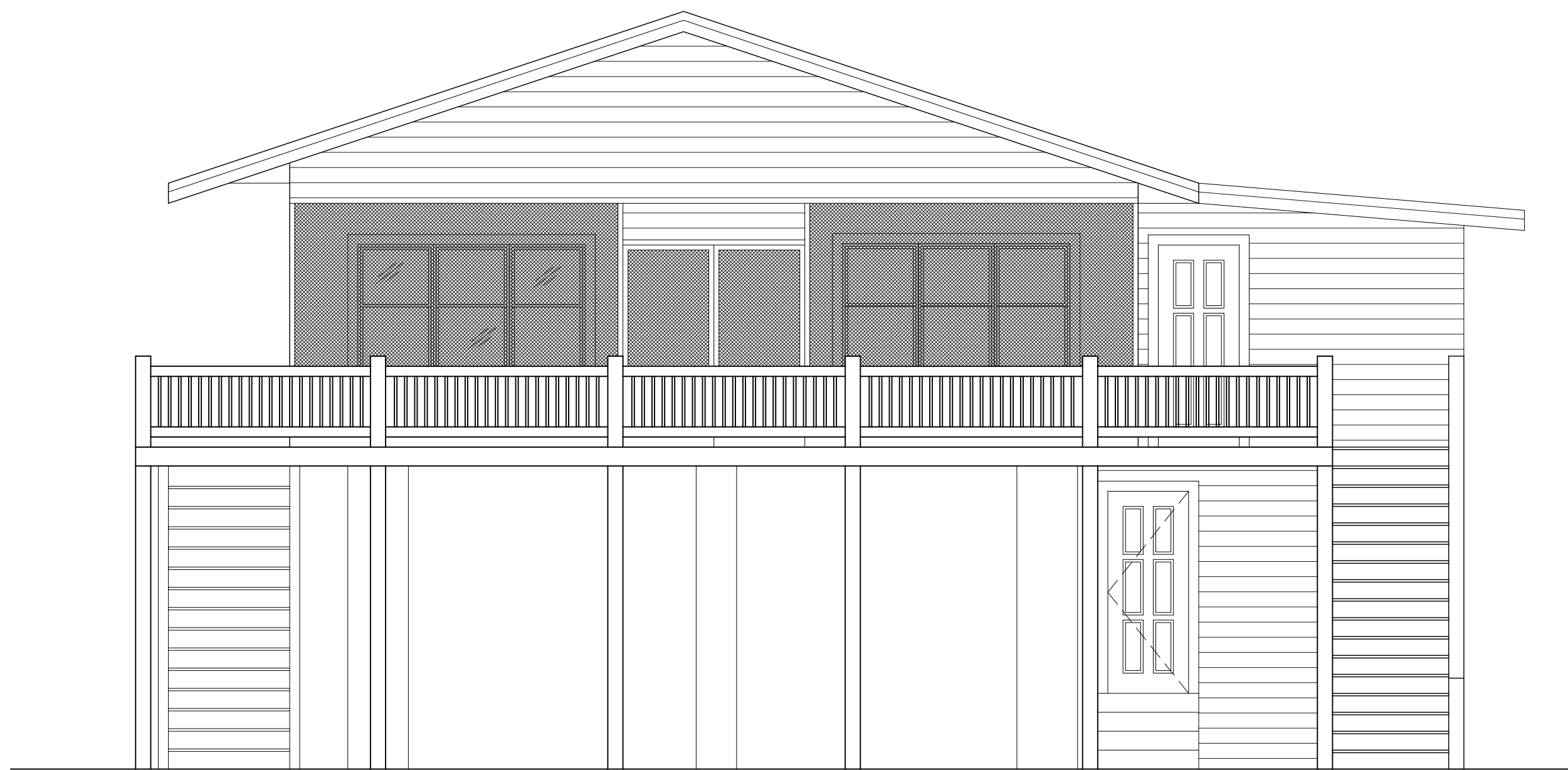
3 Rear (South) Elevation - Existing Scale: 1/4" = 1'-0"
